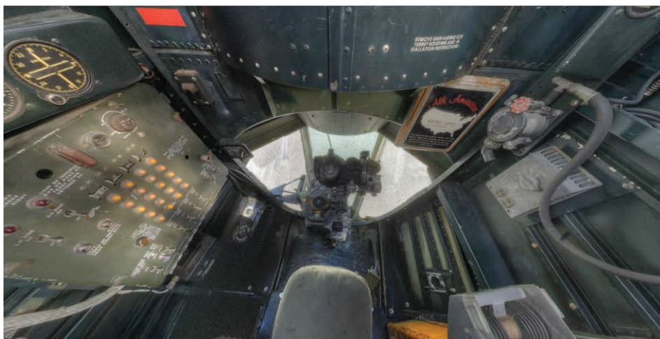
Looking Forward and Downwards to the Bombardier's Position and the Top Secret Norden Bombsight. The Nose Gunner Position Is Just Above the Bombardier Behind the Riveted Metal Bulkhead.
