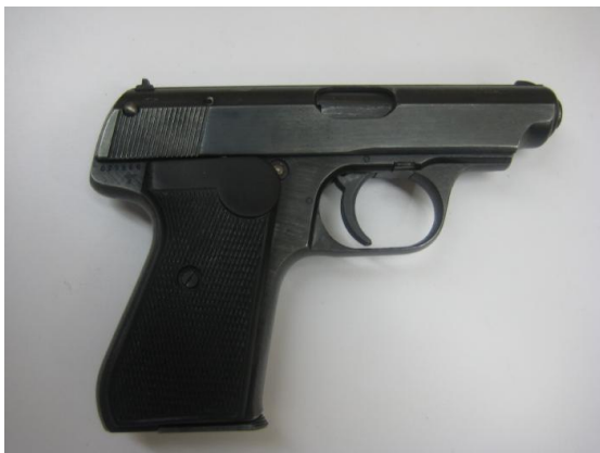
George Hofmann's "booty" included a Sauer & Sohn 38H, 0.32ACP (7.65MM) double automatic pistol and magazine. The Sauer 38H or often just H was a small semi-automatic pistol made in Nazi Germany from 1938 until just after the end of World War II by J. P. Sauer & Sohn, then based in Suhl, Germany. The "H" in the model number denotes "hammerless"—the pistol uses an internal hammer.
