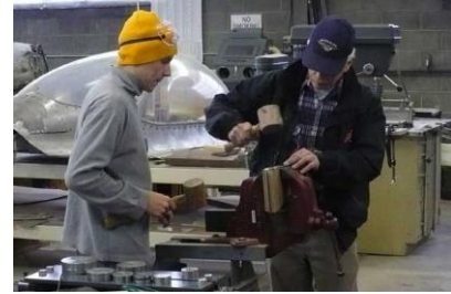
... wooden hammers bend to shape, and ...
