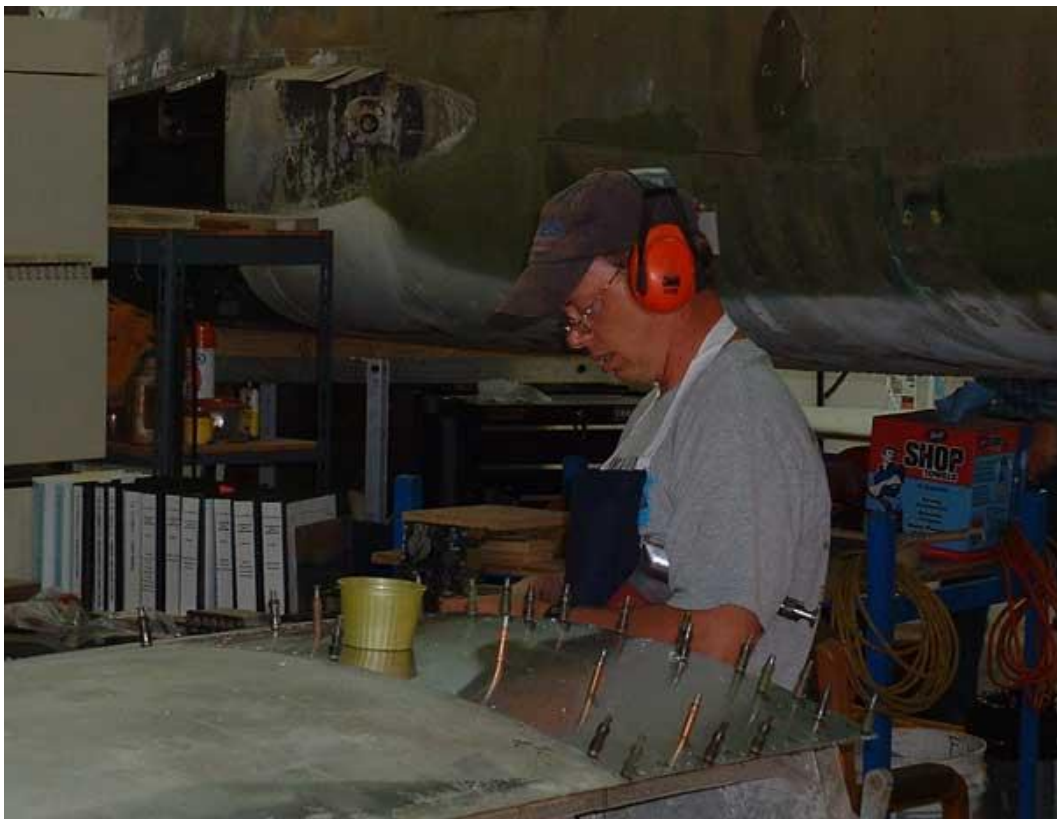
MAPS Member Kent patching one of the B-26's clamshell bomb bay doors ♦ photo ♦ James Kohan
