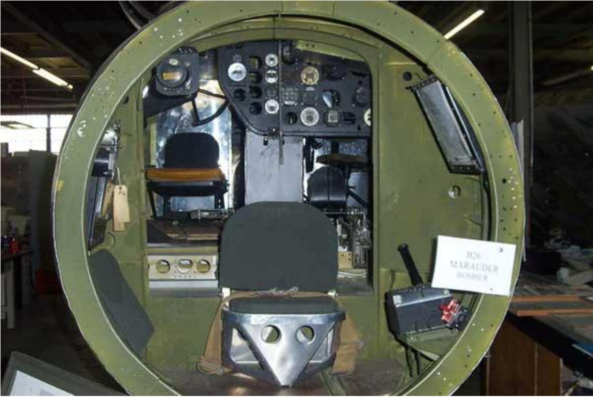
Nose compartment of the B-26. Note cockpit layout and limited access ♦ photo ♦ Gary Haught
