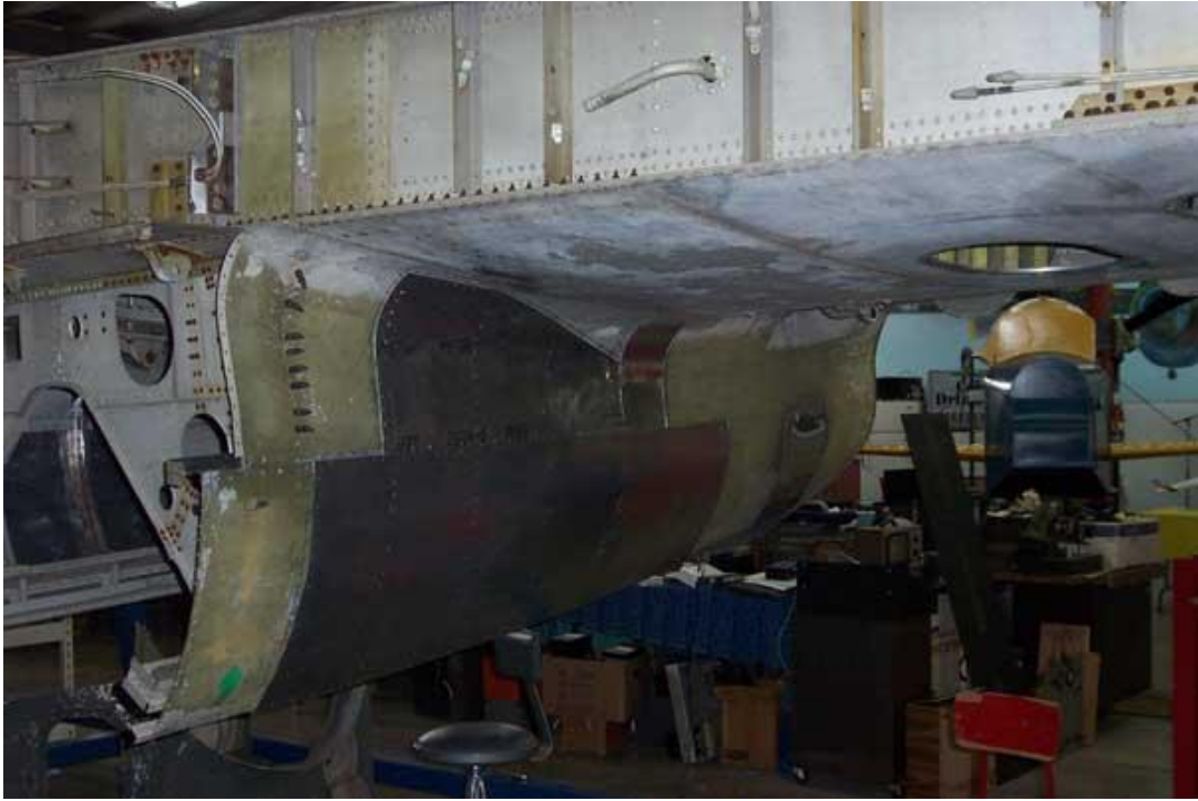
B-26 engine nacelle exterior - ALL DONE! Most of the cleco's are gone ♦ photo ♦ Gary Haught
