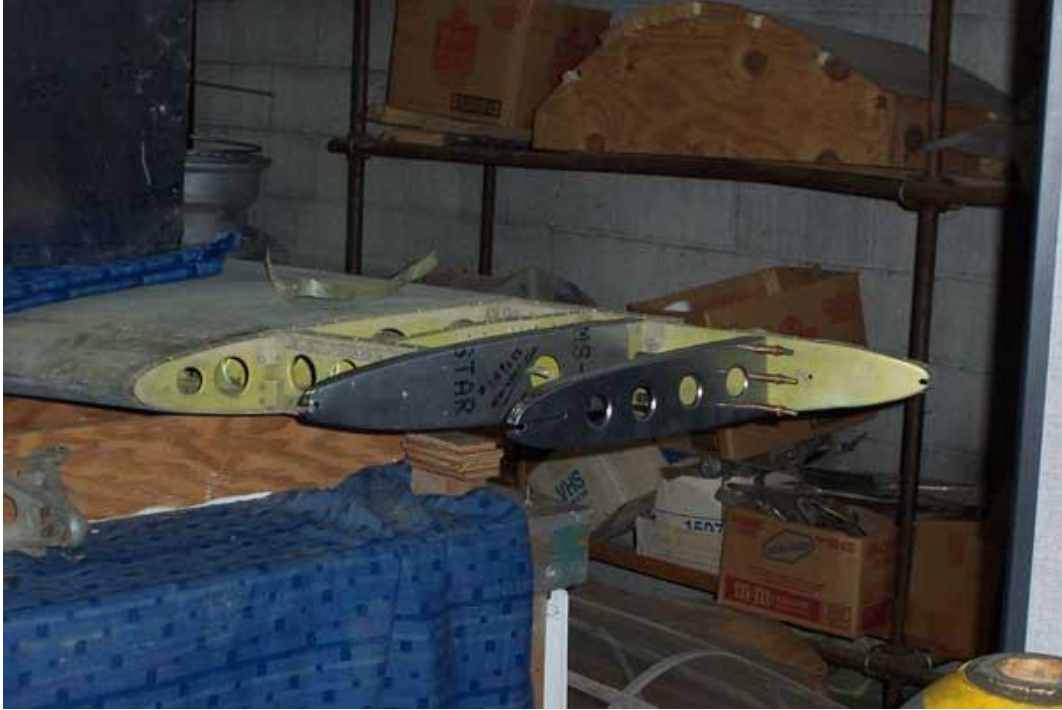
New ribs to go under the rebuilt stabilizer end ♦ photo 0000" size="1">"1"> ♦ James Kohan
