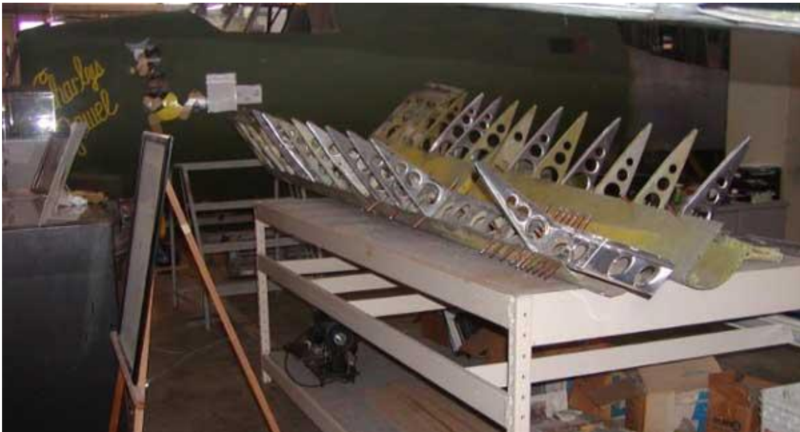
B-26 aileron ribs starting to go back on the aileron ♦ Photo ♦ Rick Willamon
