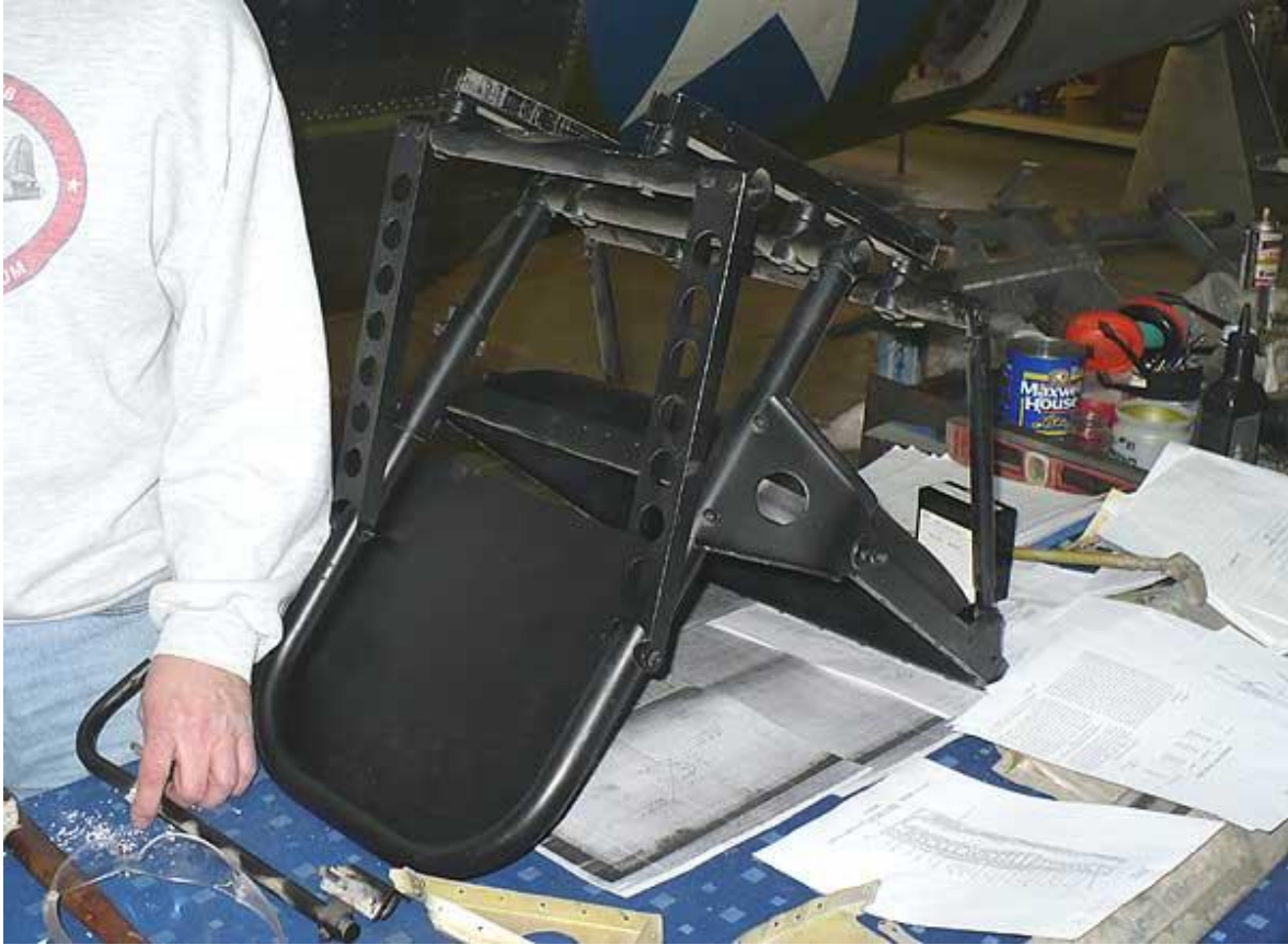
Restoration work on the B-26 co-pilot's seat. The co-pilots seat ran on rails, to allow the Bombardier to gain access to the nose compartment. The last photo on this page shows (at left) the still-in-progress seat in place in the aircraft. ♦ Photos ♦ James Ko ♦ Photos ♦ James Kohan
