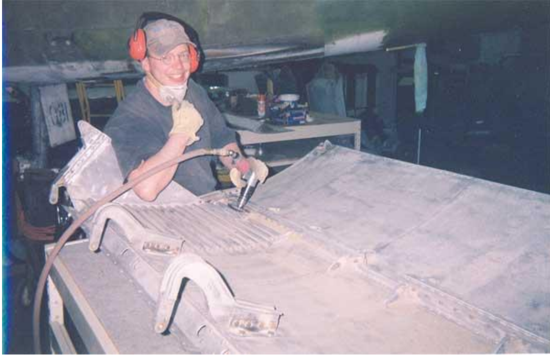
MAPS Member Kent patching one of the B-26's clamshell bomb bay doors ♦ photo ♦ Steve Satchell
