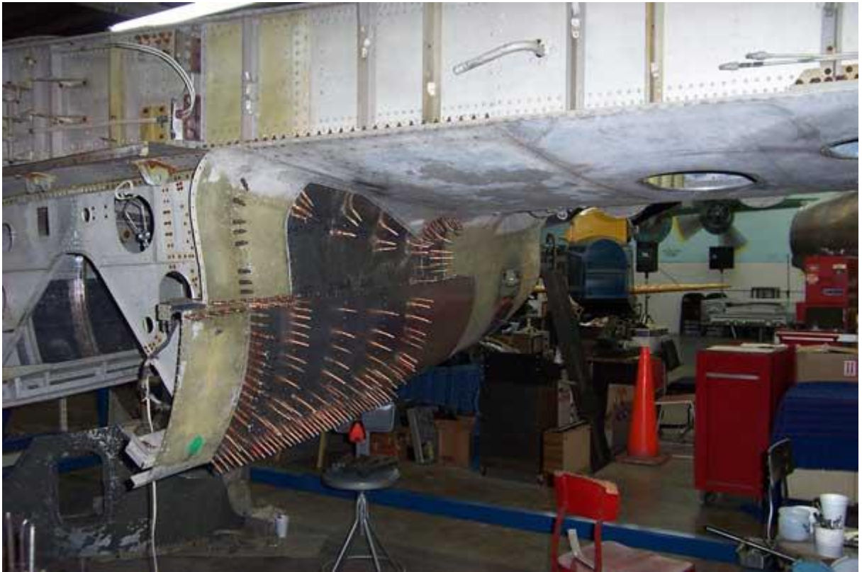
B-26 engine nacelle - Cleco's are holding the pieces together until riveting ♦ photo ♦ Gary Haught
