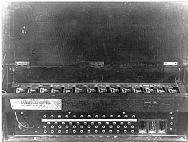
The SIS used this analog of the Japanese Purple machine to decipher Japanese diplomatic messages in 1940.
