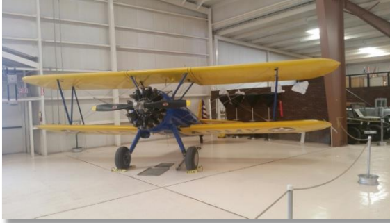
The Stearman (Boeing) Model 75 is a biplane used as a military trainer aircraft, of which at least 10,626 were built in the United States during the 1930s and 1940s. It was a popular trainer used by WWII fighter pilots.
