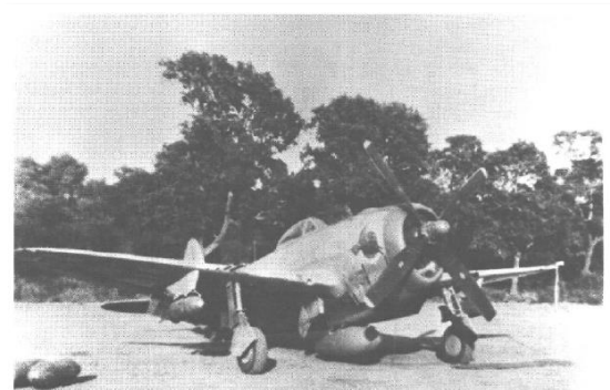
A Republic P-47D Thunderbolt shown with two 500-lb bombs and an external fuel tank, a typical offensive load carried in the 1944 campaign across France.
