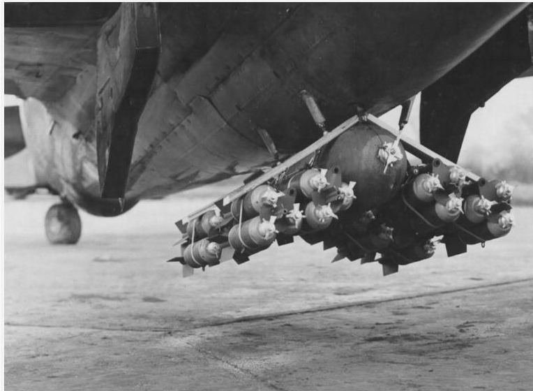
© Fold3 An example of a typical fragmentation bomb mounted on a P-47 Thunderbolt; these devices were used in dive-bombing missions against airfields in Spring 1944, with varying results.
